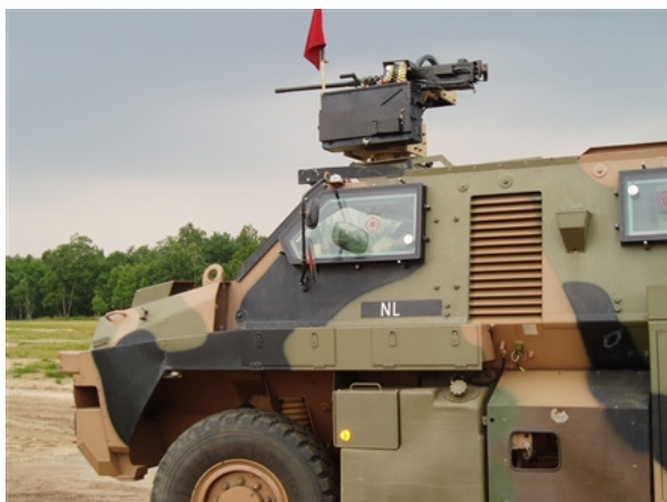
A Raven/Crows system seen integrated on a Netherlands Bushmaster vehicle during field testing. Starting in August, this configuration will enter service with Dutch forces in Afghanistan. Photo: Royal Netherlands Army
